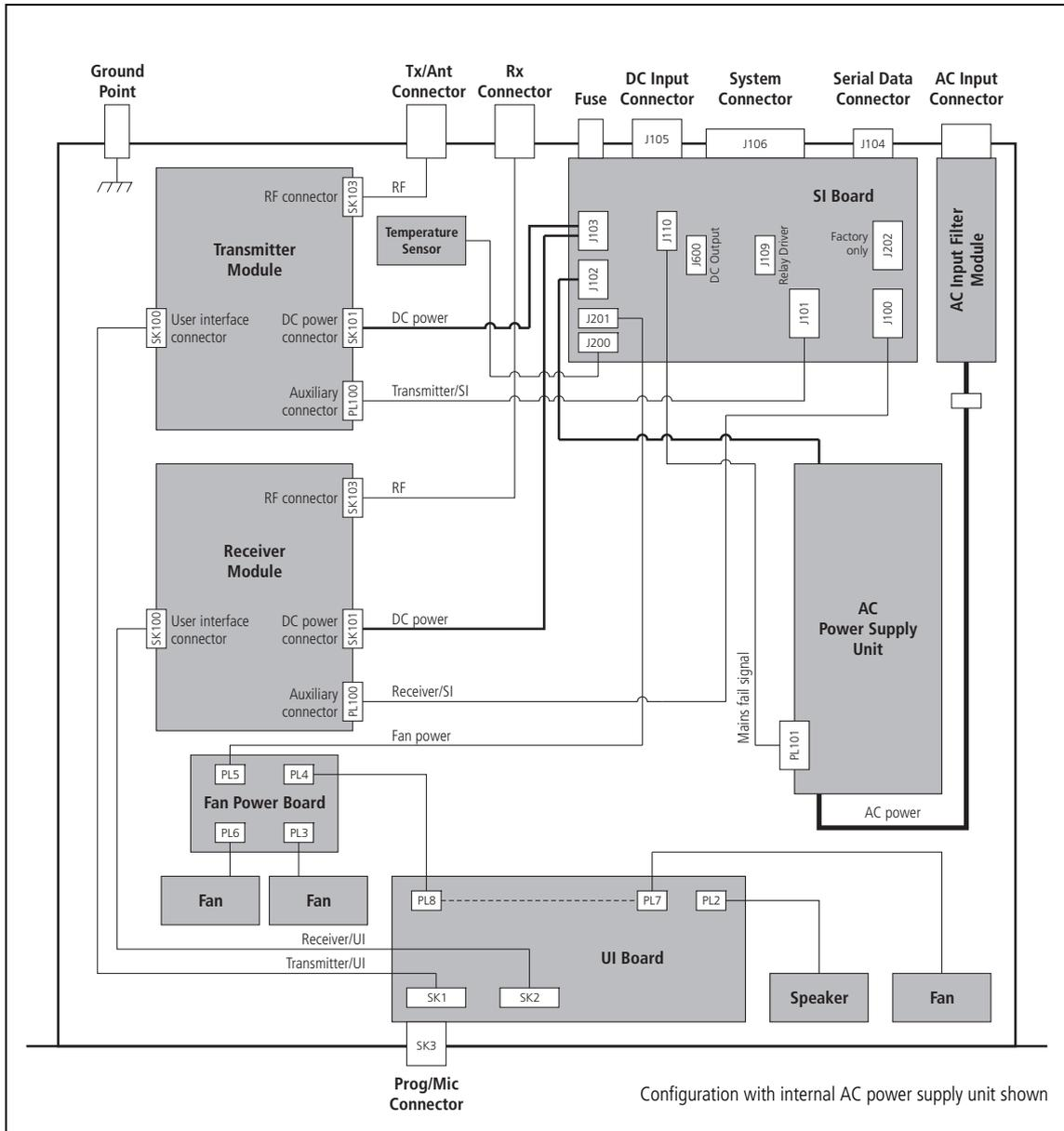
For information on the factory connector and the internal options connector of the transmitter and receiver, refer to the PCB information.
