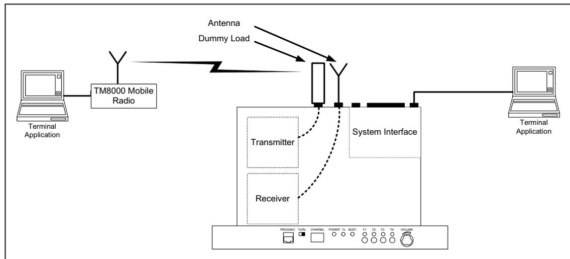
The correct operation of the base station as an RF modem can be verified by transferring text files between the two PCs.
