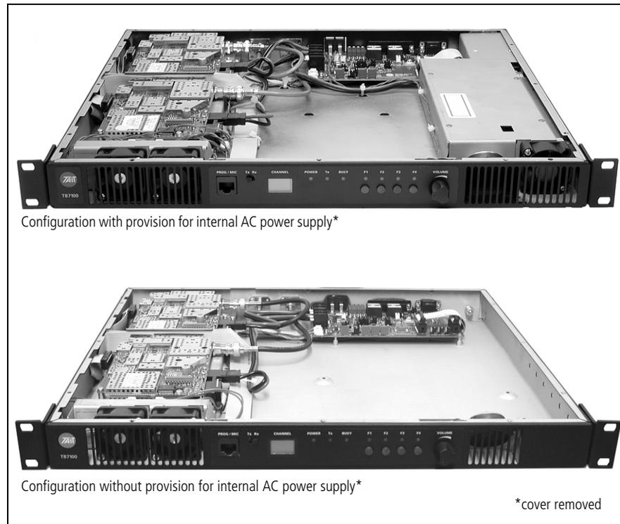
The TB7100 is a software and hardware link-configured base station which is designed for operation in a large variety of standard frequency ranges. It makes extensive use of digital and DSP technology. Many operating parameters such as channel spacing, audio bandwidth and signalling are controlled by software.
