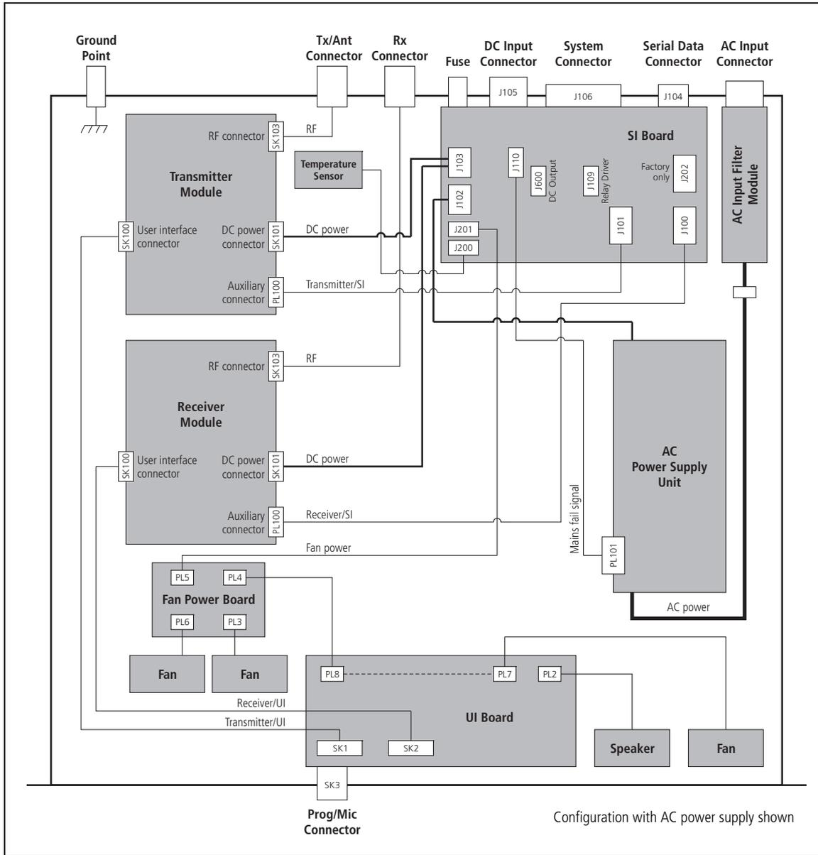
The block diagram illustrates the main inputs and outputs for power, RF and control signals, as well as the interconnection between modules:
