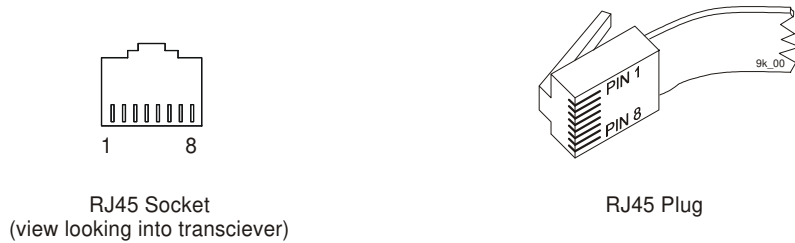
Figure A.1 SRM9000 RJ45 Pinout (S1)
