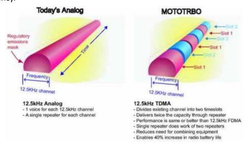
TDMA thereby offers a straightforward method for achieving 6.25kHz equivalency in 12.5kHz
