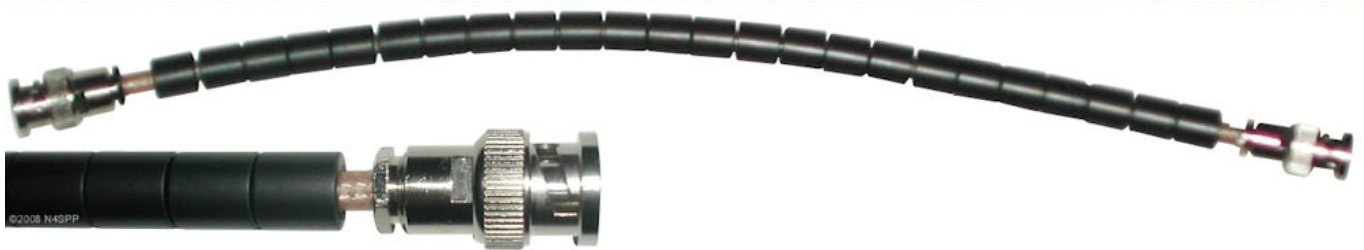
My W2DU-style common-mode current choke
